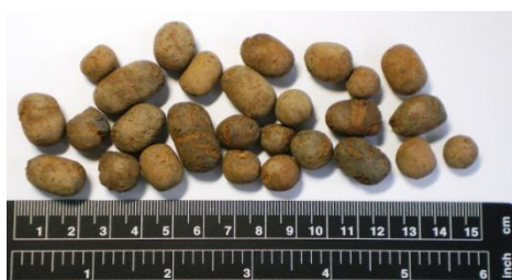
Figure 3: Appearance of sintered sedimentary LWA
