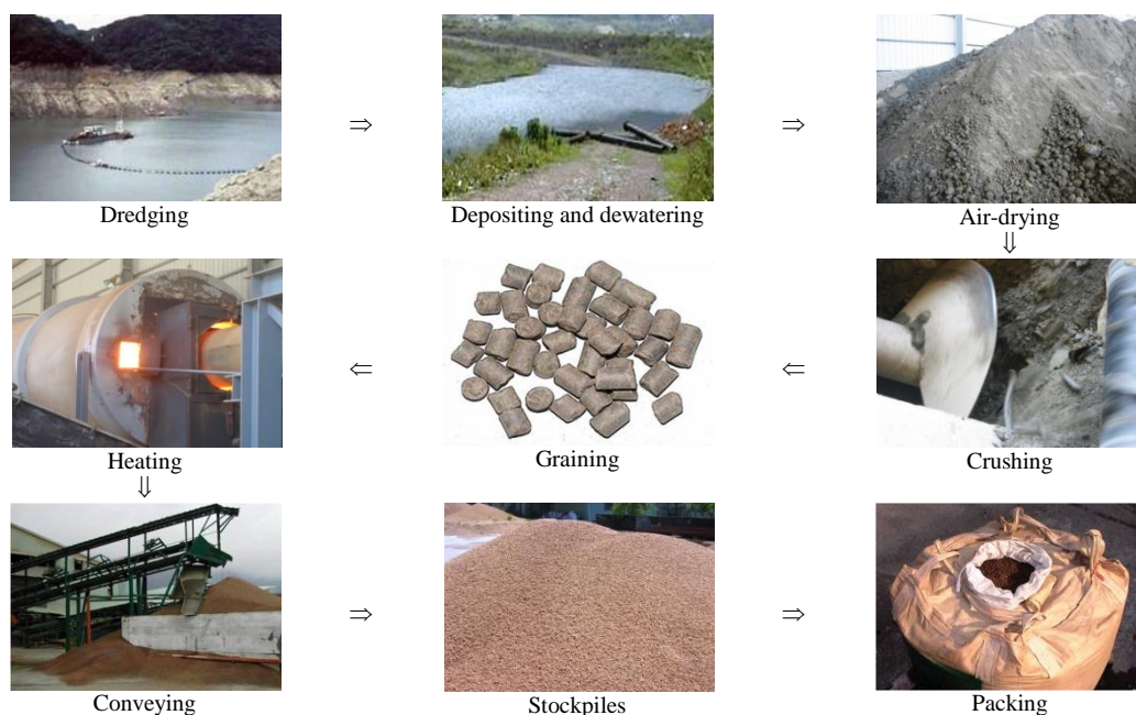
Figure 2: The flow diagram of the manufacturing processes for the sintered sediment LWA
